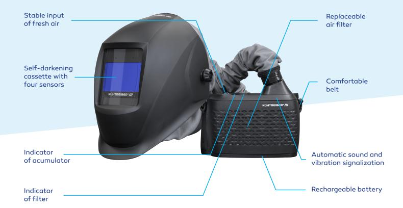
This welding mask Kühtreiber Freflow V1 is designed for welding by arc method (MMA, MIG/MAG, TIG DC and TIG AC), welding by micro-plasma, welding by gas and plasma-cutting. Because of the grinding funcition is ready for using to protect of the face and head of the welder during grinding.
